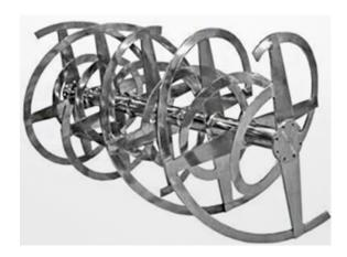
**Ribbon Blender** comprises of a U-shaped horizontal trough and a specially designed Double Helical Ribbon Agitator rotating within. Ribbon Blenders are based on a proven agitator construction that provides a triple mixing action ensuring fast, efficient blending. The dimensions and configuration of the ribbons are carefully balanced to provide a movement of material within the container that avoids dead spots and gives rapid product discharge.
