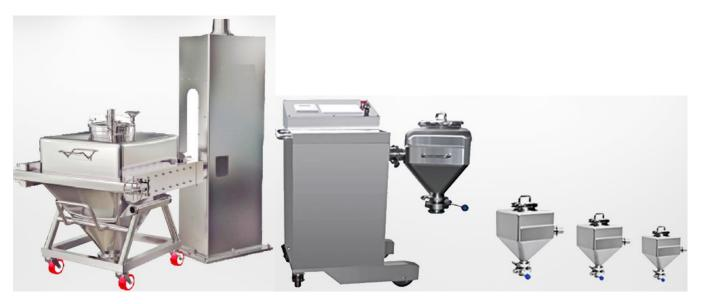
Bin blenders are used mainly for blending of dry powders for tablet and capsule manufacturing process, which facilitates better flow for tablets and capsules. This is a closed contained, totally dust free single step transfer system. It can handle more than one size of container (Bin)
