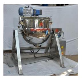
Jay Pharma Binder Preparation Vessel (Starch Paste Preparation Kettle) has been designed uniquely for optimal mixing efficiency so as to ensure a homogeneous mix. The special stirrer in the vessel has been designed to create vortex inside the solvent which enhances the desired solubility of pharmaceutical binder solute into the various solvents.
